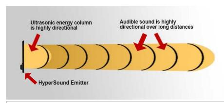
HyperSound generates an ultrasonic energy beam that is highly directional, and converts to audible sound in the air. The length of the column determines the directionality at audio frequencies. This sound is directional over longer distances than traditional loudspeakers.
